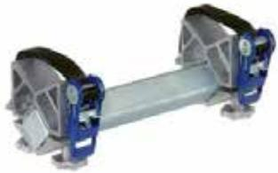
Pipe clamps keep the PE pipes and fittings locked in position during the welding and cooling period, preventing pullout and movement that could compromise leaktightness of the joints.
