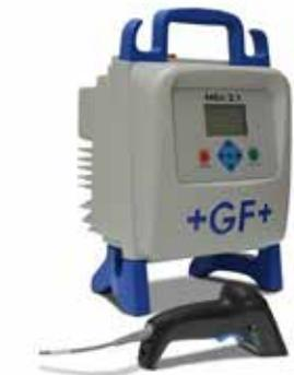
A fully automatic electrofusion machine with barcode reader realises reliable joints coupling after coupling, without manual configuration and intervention. The entire welding process is guided step by step via the graphical colour display. The weld protocols are internally stored and can be exported on a USB stick for archiving purposes.
